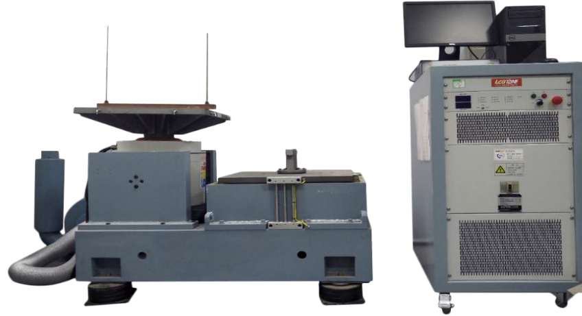
Vibration Test Equipment
