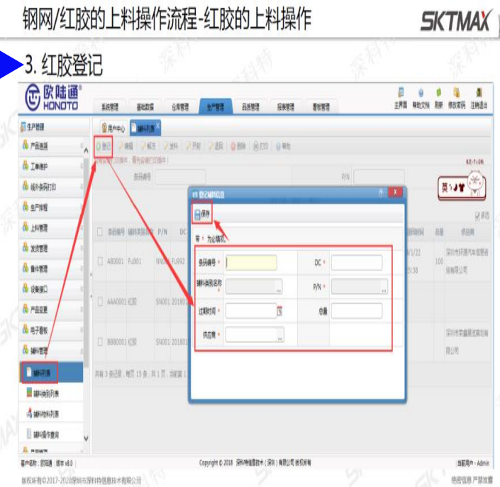
MES system controls the use, storage time, return temperature time and on-line time of solder paste
